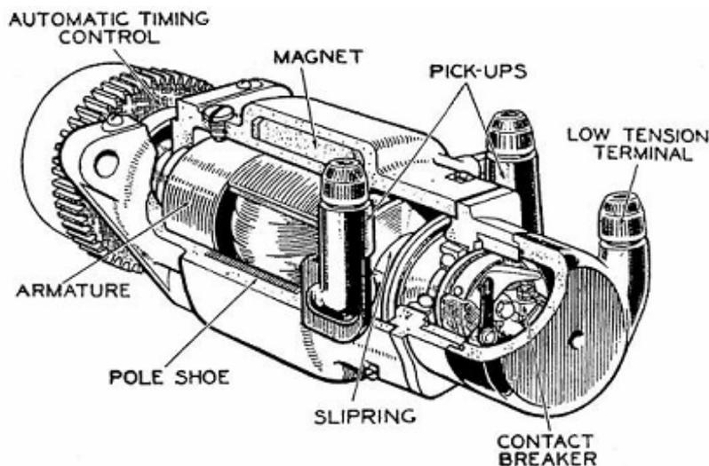
Type: K2F—For horizontally opposed or vertical twin engines.
