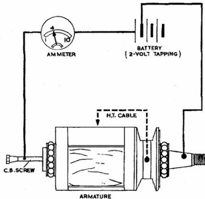
**Testing Primary & Secondary Windings**
