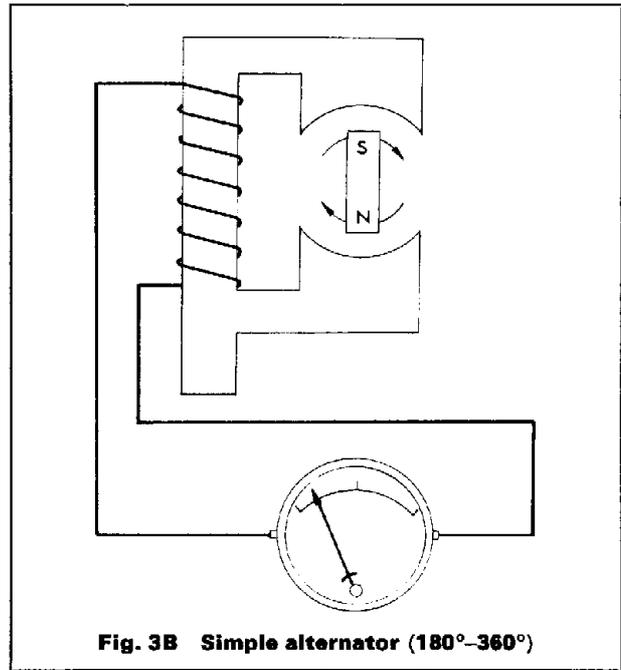
Fig. 3B Simple alternator (180°-360°)
