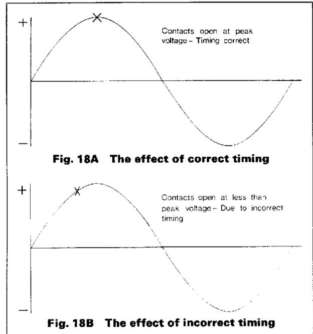
will not open at the peak of the voltage curve, see Fig. 18 (B) and consequently the spark will be weak. REMEMBER, IGNITION TIMING IS CRITICAL.
