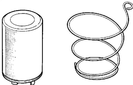
Fig. 34 Capacitor model 2MC and mounting spring
