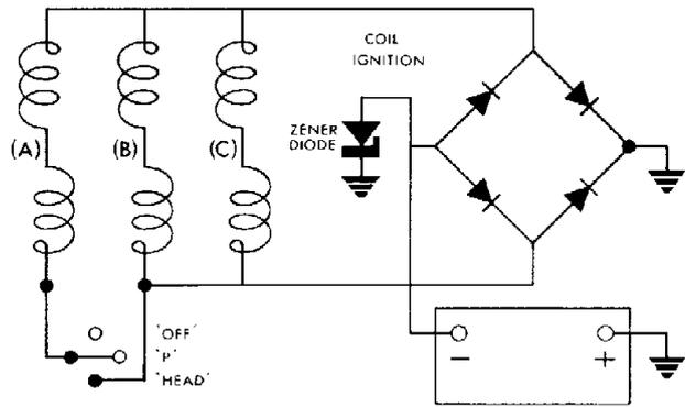
Fig. 51A Charging circuit showing Zener diode connection
