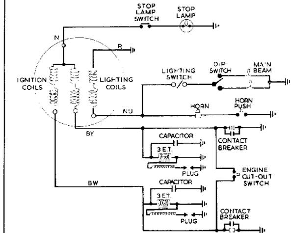
Fig. 21 A.C. ignition circuit for twin contact motor cycles
