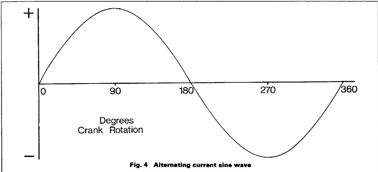
Fig. 4 Alternating current sine wave
