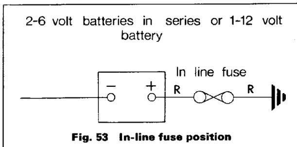
Fig. 53 In-line fuse position
