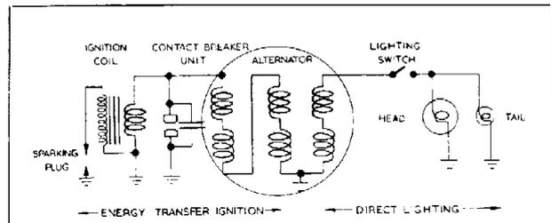
Fig. 20 A.C. ignition circuit for single cylinder motor cycles
