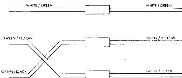
Fig. 56 Alternator connections for coil ignition motor cycles
