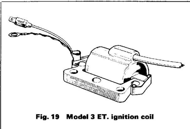
Fig. 19 Model 3 ET. ignition coil
