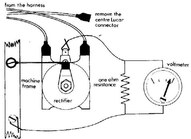
Fig. 68 Rectifier test in position
