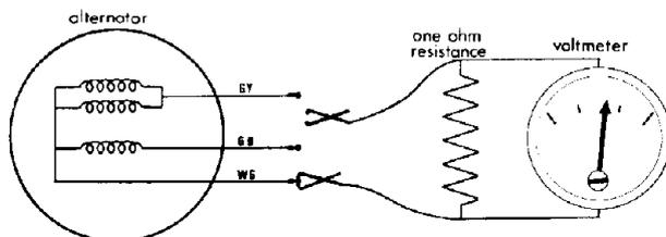
Fig. 67 Alternator output test
