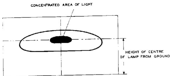
Fig. 41 Headlight adjustment
