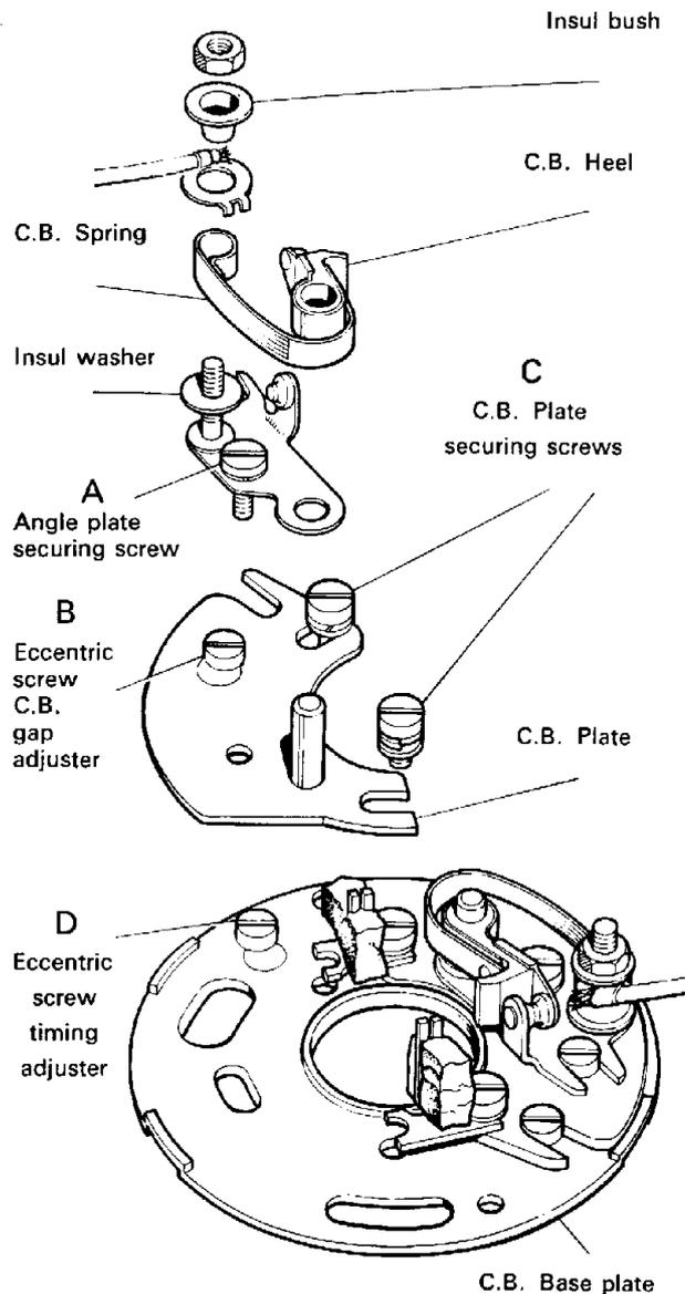
Fig. 28 Contact breaker model 6CA
