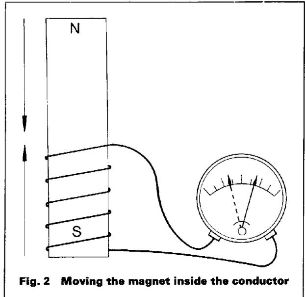
Fig. 2 Moving the magnet inside the conductor
