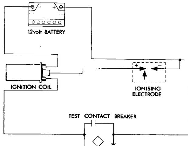
Fig. 75 Ignition coil bench test circuit
