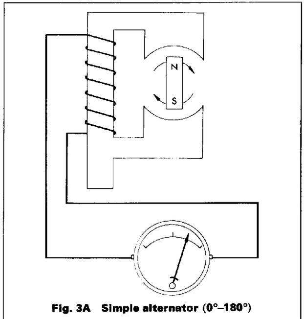
Fig. 3A Simple alternator (0°-180°)
