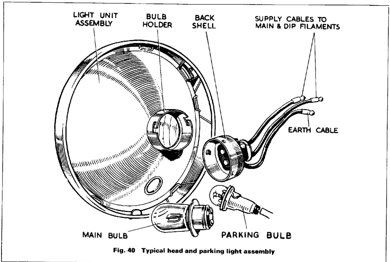
Fig. 40 Typical head and parking light assembly
