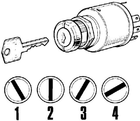
Fig. 48 Ignition/Light switch model 149SA
