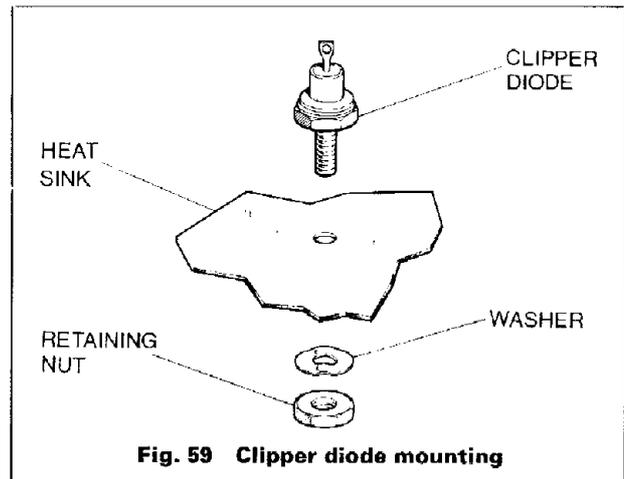
Fig. 59 Clipper diode mounting
