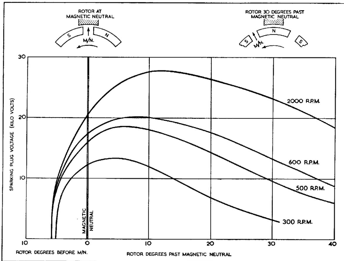
Fig. 22 The effect of magnetic timing on plug voltage at various rev/min
