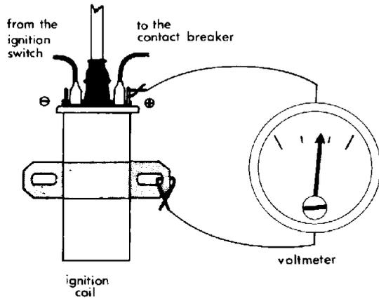
**Fig. 71 Coil and contact breaker circuit test**
