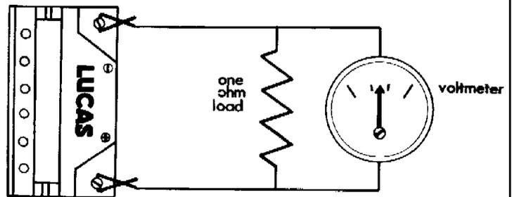
Fig. 65 High rate discharge test
