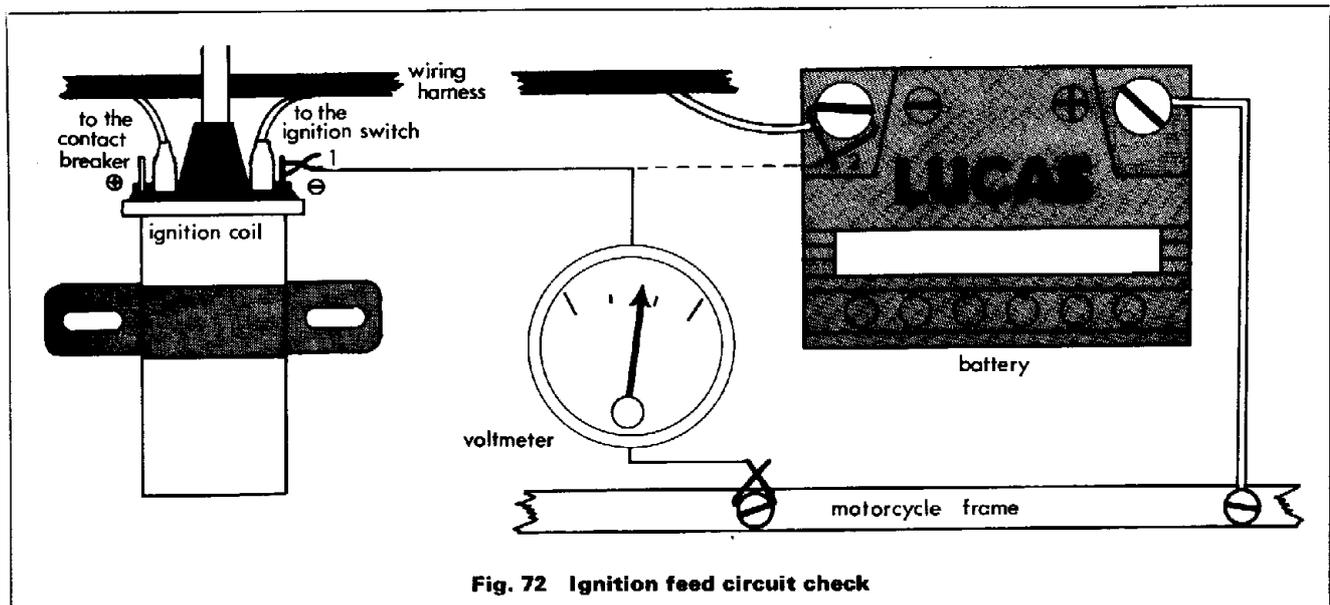
**Fig. 72 Ignition feed circuit check**
