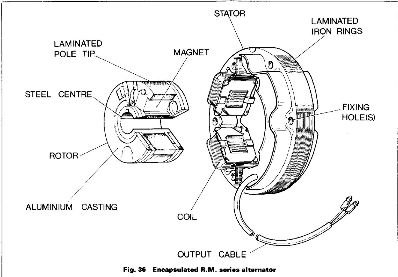
Fig. 36 Encapsulated R.M. series alternator
