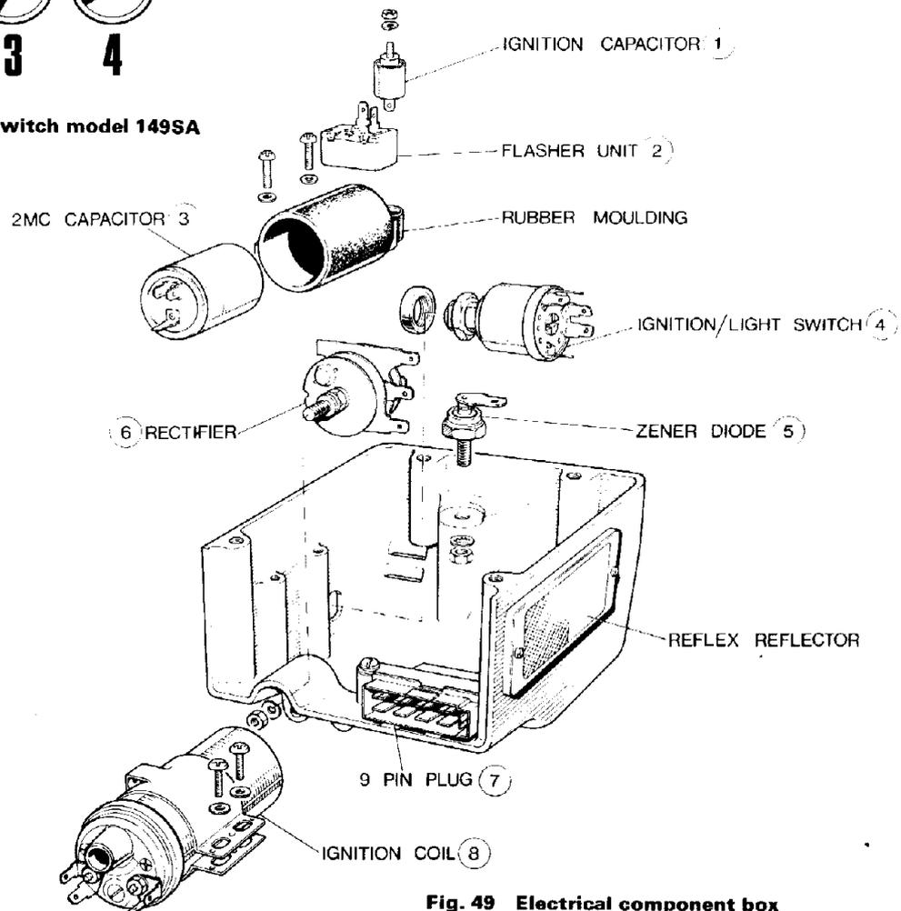
Fig. 49 Electrical component box
