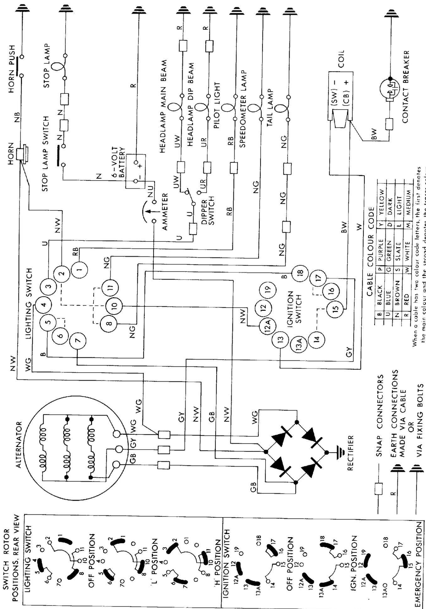
**Fig. 77 Typical 6 volt system with 88SA ignition and light switches**
