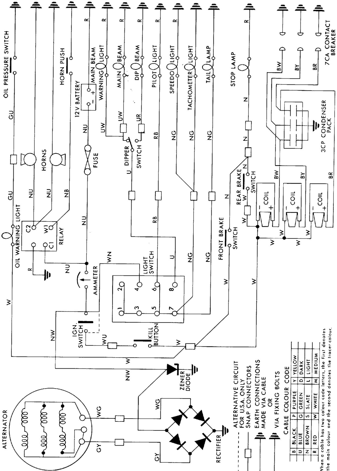
Fig. 83 Typical 12 volt system for three cylinder machines
