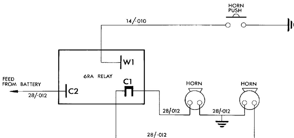
Fig. 61 Twin horn circuit
