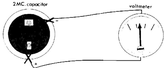
**Fig. 73 Capacitor bench test**
