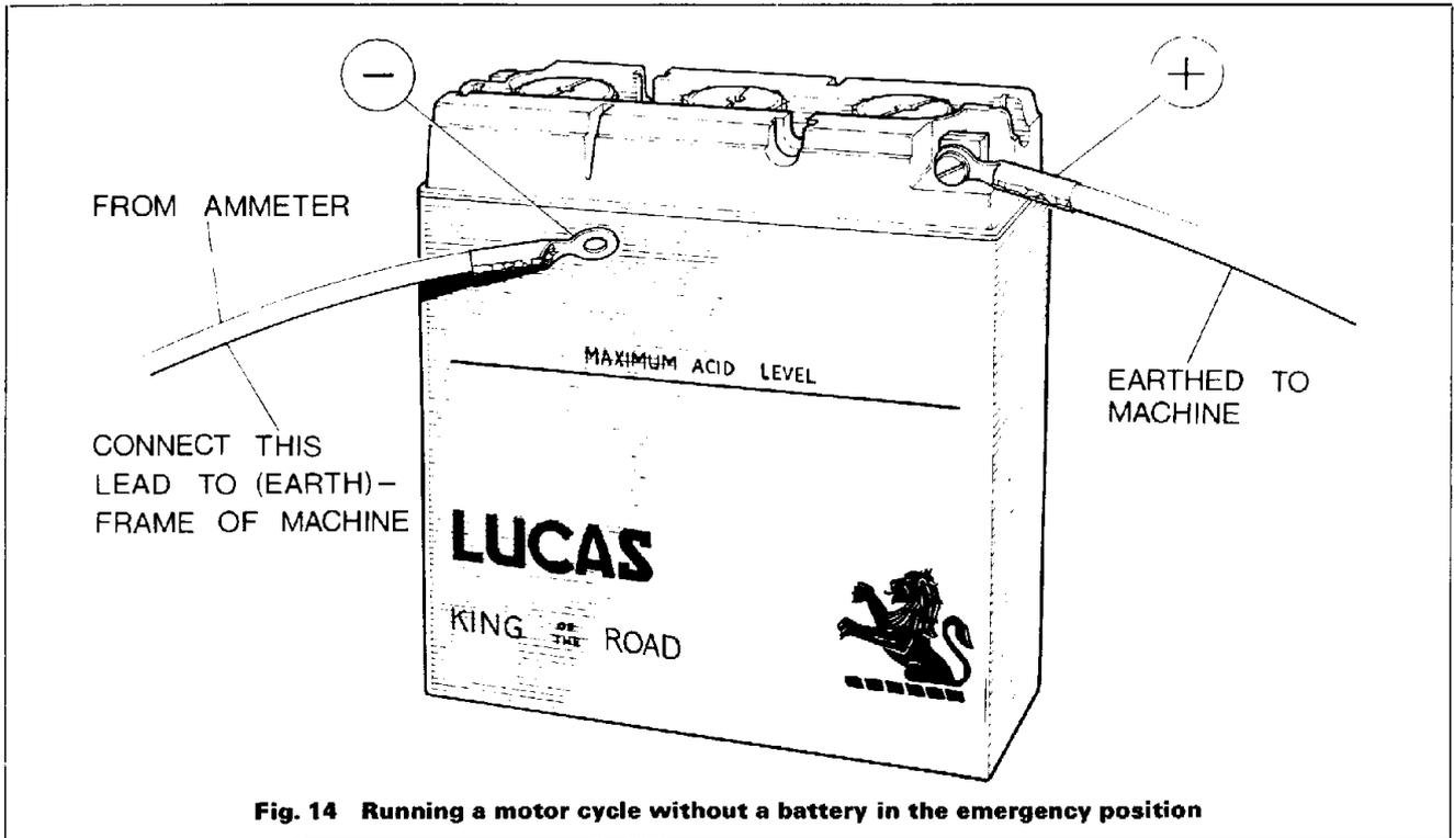
**Fig. 14 Running a motor cycle without a battery in the emergency position**
