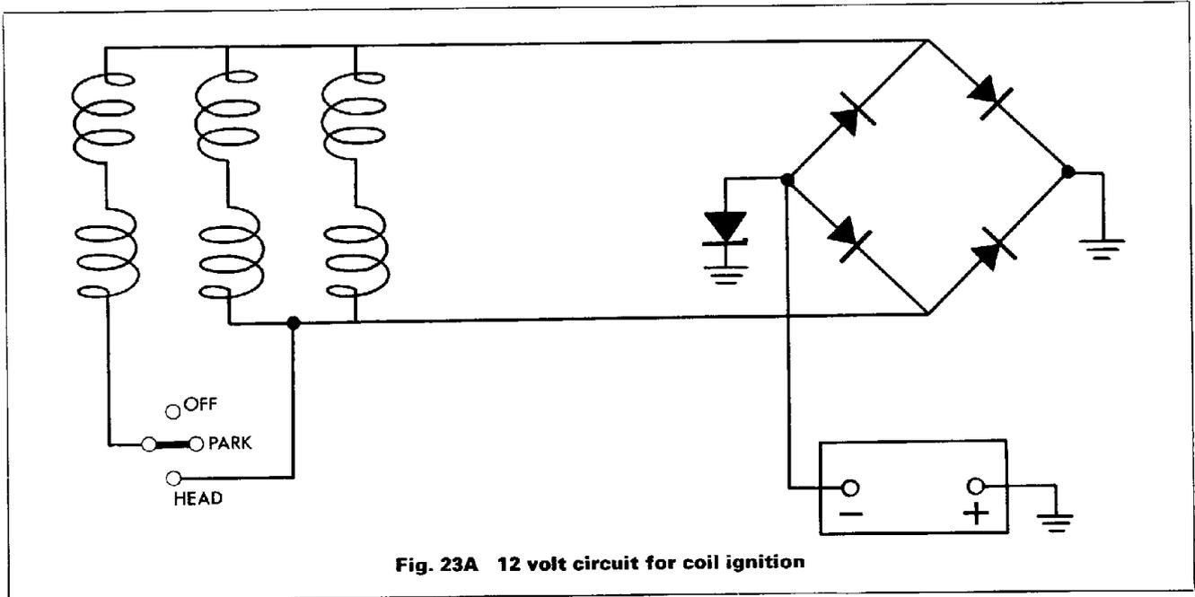
Fig. 23A 12 volt circuit for coil ignition
