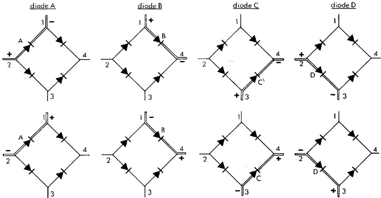
Fig. 69B Rectifier bench test (individual diode circuits)
