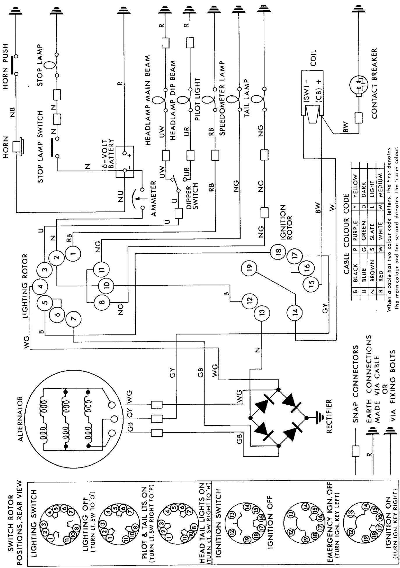
**Fig. 76 Typical 6 volt system using PRS8 switch in a single cylinder machine**
